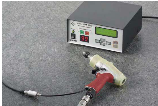
UTM-1500(CN): Connector Incorporated type By connecting the pressure sensor (external pressure sensor assembly) attached to a tool to the connector at the back of controller, the controller supplies the power and loads the analog signal.
