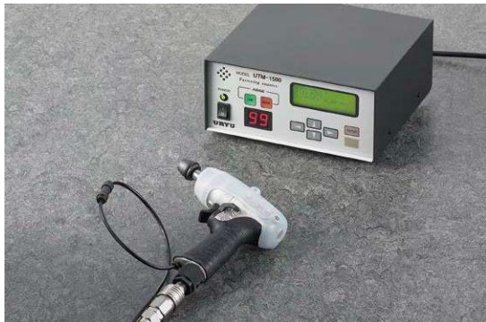
UTM-1500(PS): Pressure Sensor Incorporated type By connecting the TM signal hose from a tool to the coupler at the back of the controller, the pressure sensor incorporated in the controller converts the air pressure signal into the electric signal.
